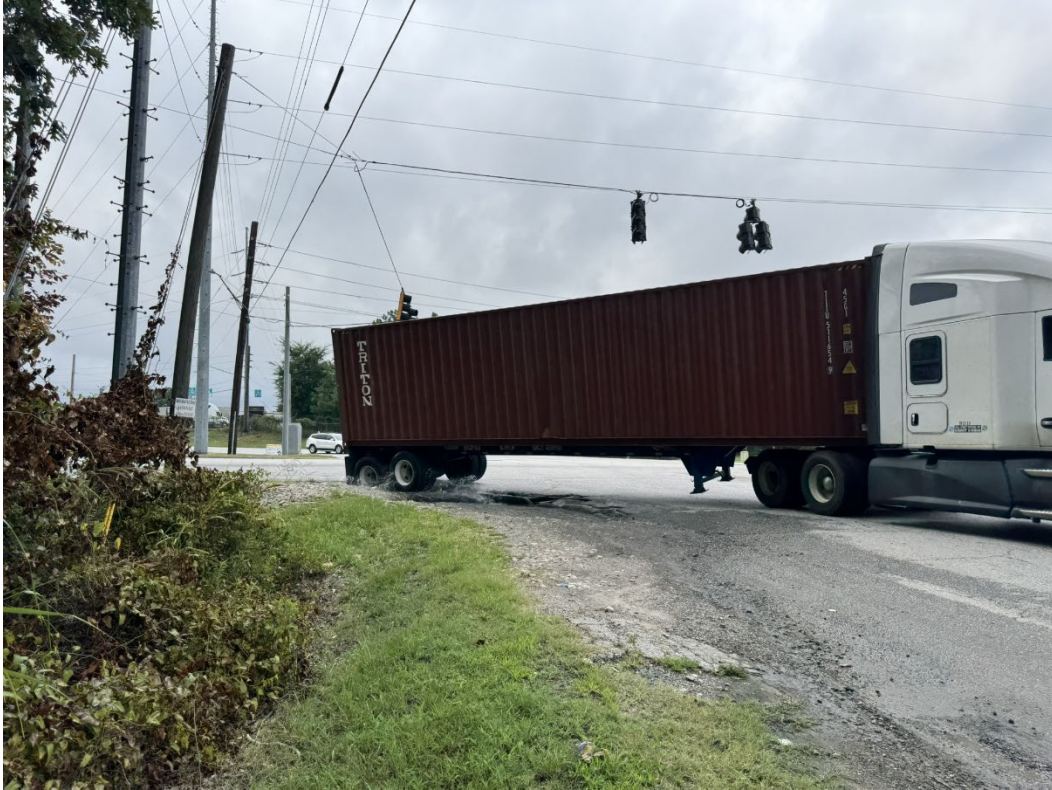
Figure 3: Truck Overtracking into Pothole Making a Southbound Right Turn
